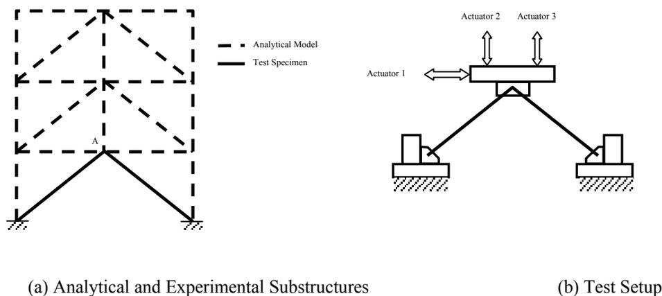
Figure 6 – Fast Hybrid Tests at the University of Colorado
