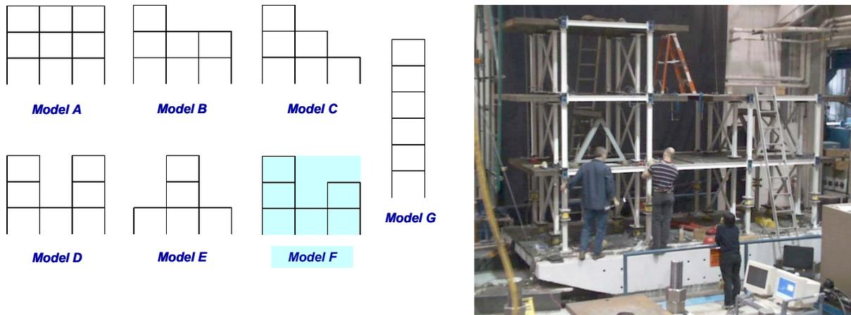
Figure 5: Reconfigurable modular structural system
