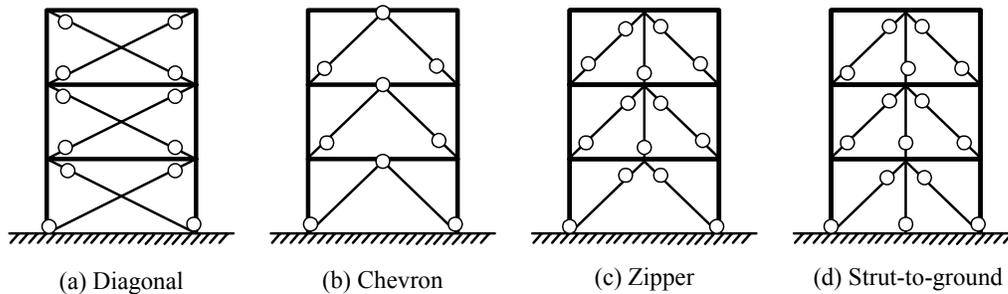
Figure 1 – Typical braced frame configurations (circles denote possible locations for energy dissipators).
