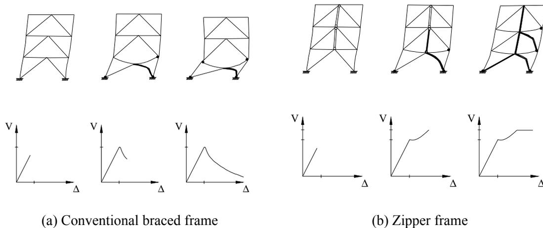
Figure 2 – Comparison of the collapse mechanism and load-displacement relationships for zipper and conventional braced frames (Khatib et al. 1988).
