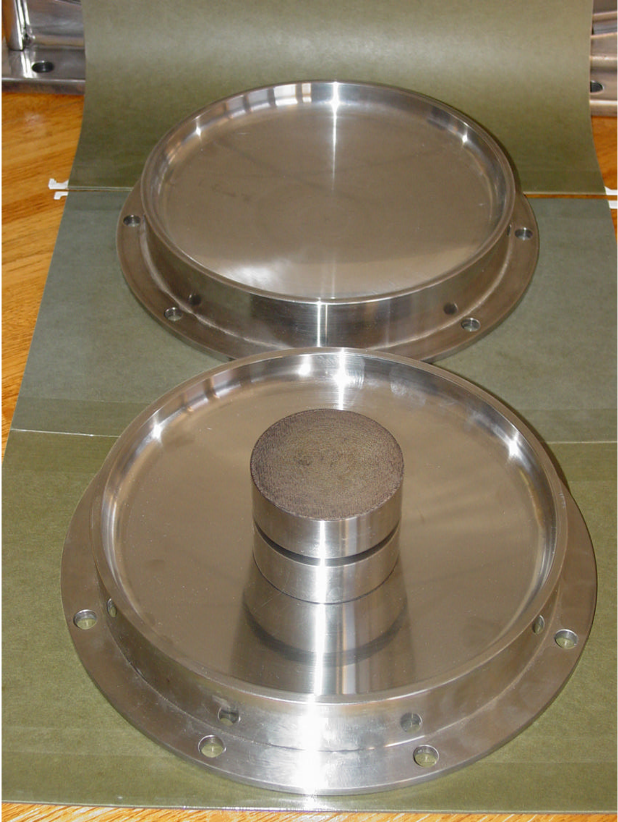
Figure 8 View of Double Concave FP Bearing
