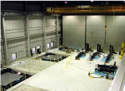
The parent platform of each shake table is 3.6 meters x 3.6 meters.
