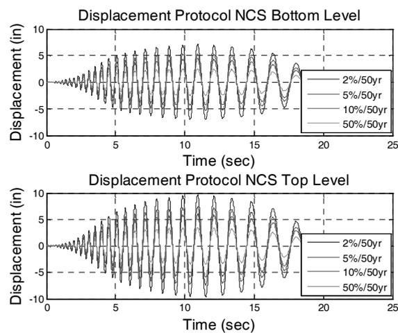
Figure 9. Displacement protocols for several seismic hazard levels.
