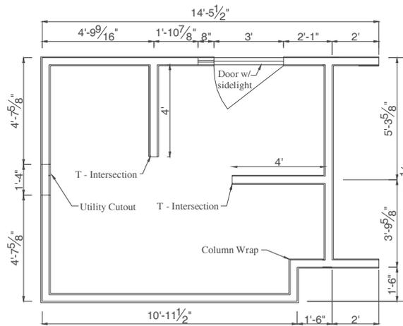
Figure 7. Geometry of specimen for the UB-NCS demonstration project (1' = 25.4 mm, 1' = 0.3048 m).
