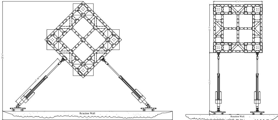
Figure 2. Plan view of bi-axial and uni-axial testing configurations (1' = 0.3048 m).
