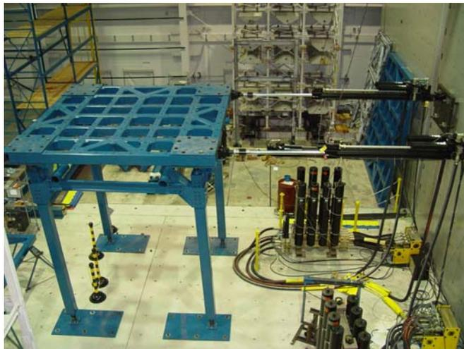
Figure 6. UB-NCS configured for single level testing.
