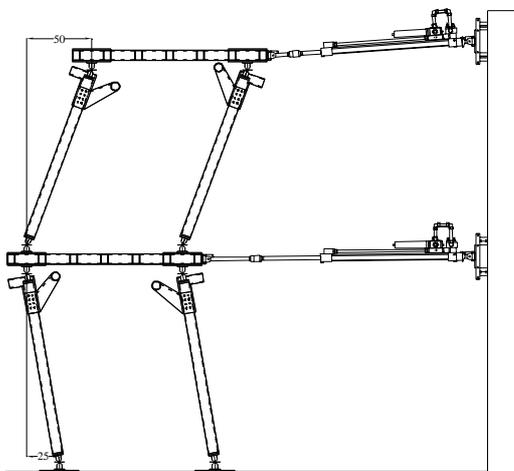
Figure 4. Deformed shape of UB-NCS 32% inter-story drift at top level. (1" = 25.4 mm).
