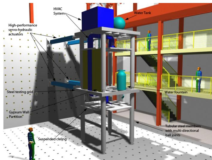
Figure 1. Nonstructural Component Simulator.
