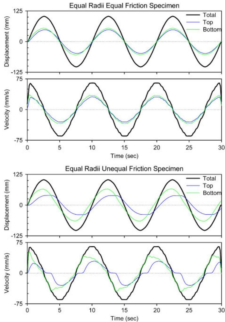
Figure 9. Recorded histories of displacement and velocity for specimen with equal radii.
