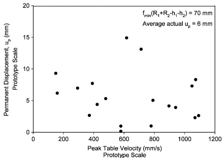
Figure 13. Actual permanent displacements (in prototype scale) measured after 19 unidirectional shaking table tests.
