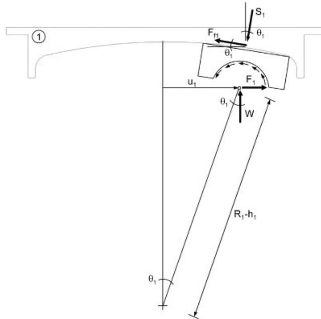
Figure 3. Free body diagram of slider on upper concave surface in the deformed configuration.
