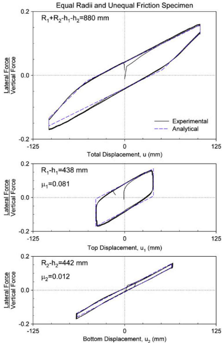
Figure 8. Comparison of experimental and analytical hysteresis loops for specimen with equal radii and unequal friction.
