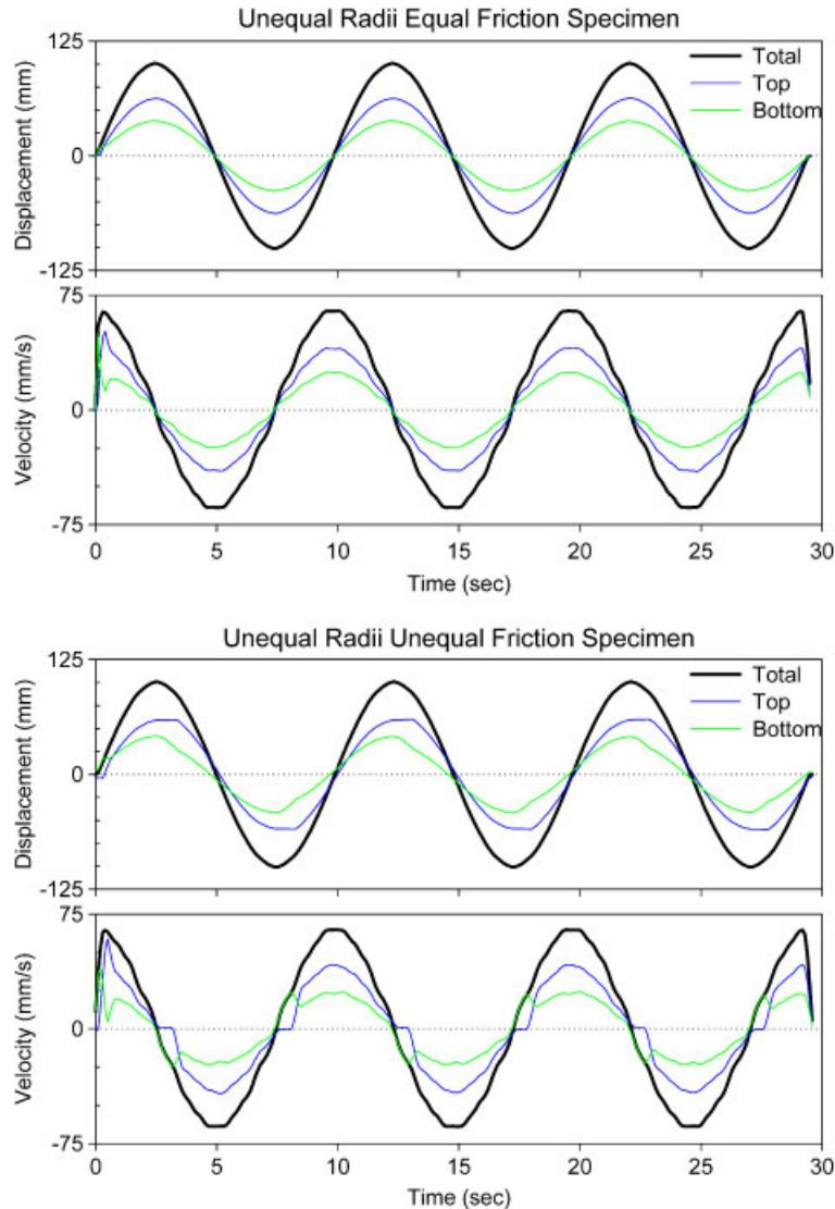
Figure 12. Recorded histories of displacement and velocity for specimen with unequal radii.
