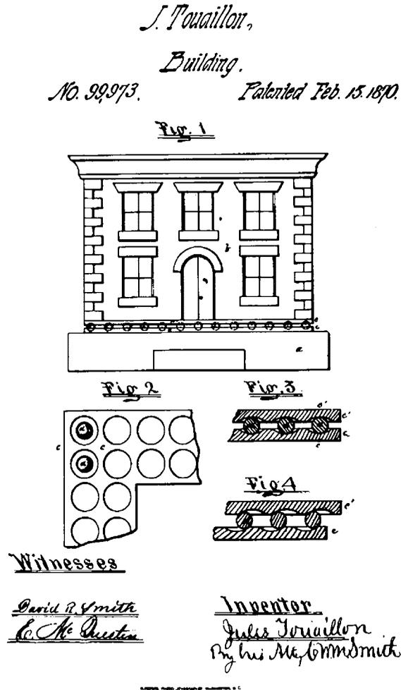
Figure 1. Jules Touaillon's original patent for a double concave rolling ball bearing.
