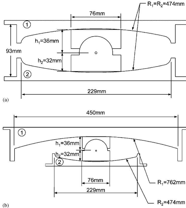
Figure 6. Specimens with concave surfaces: (a) having equal radii of curvature; and (b) unequal radii of curvature used in characterization testing.
