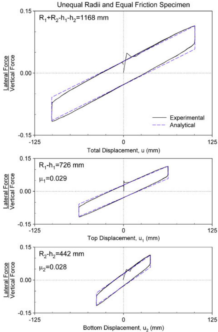
Figure 10. Comparison of experimental and analytical hysteresis loops for specimen with unequal radii and equal friction.
