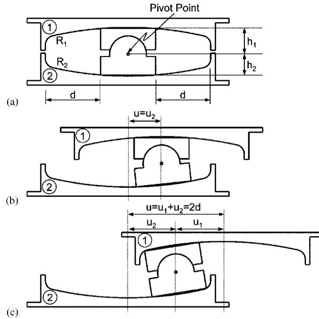
Figure 2. Section through centre of DCFP bearing at various stages of motion.
