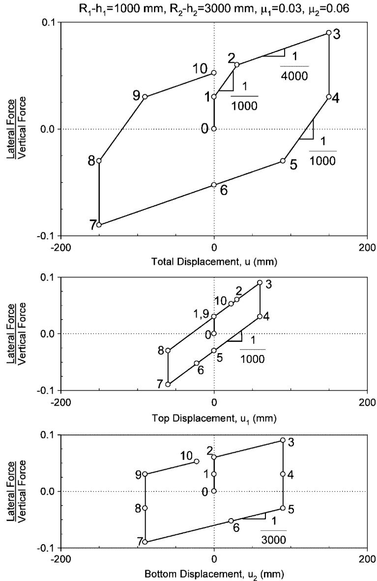
Figure 5. Example hysteresis loops for a configuration of DCFP bearing having unequal radii of curvature and unequal coefficients of friction.
