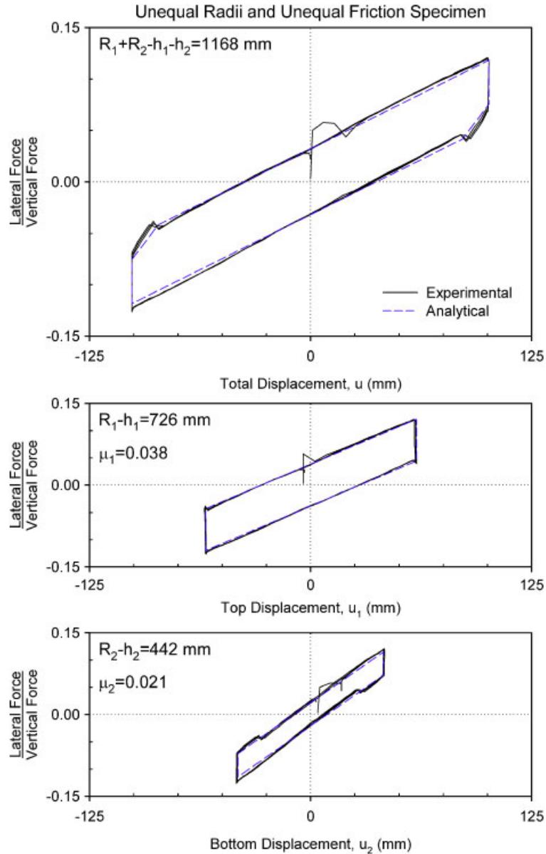
Figure 11. Comparison of experimental and analytical hysteresis loops for specimen with unequal radii and unequal friction.
