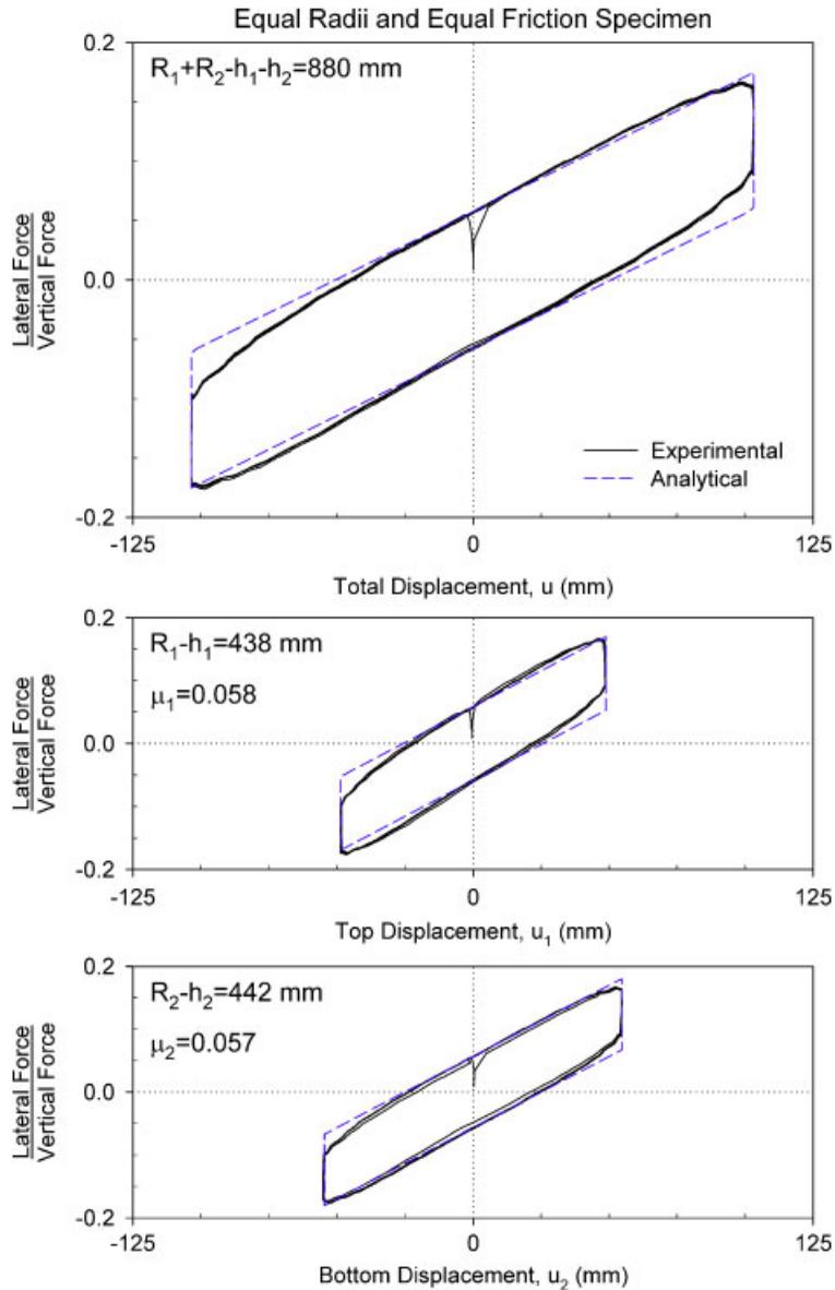
Figure 7. Comparison of experimental and analytical hysteresis loops for specimen with equal radii and equal friction.
