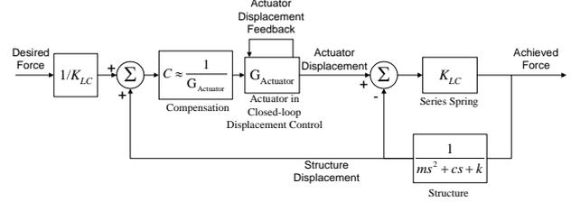
**Figure 4:** Block diagram of proposed force control
