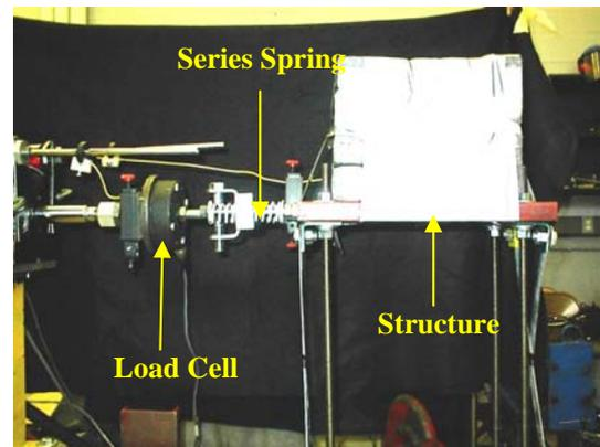
**Figure 5:** (a) Small scale force control setup
