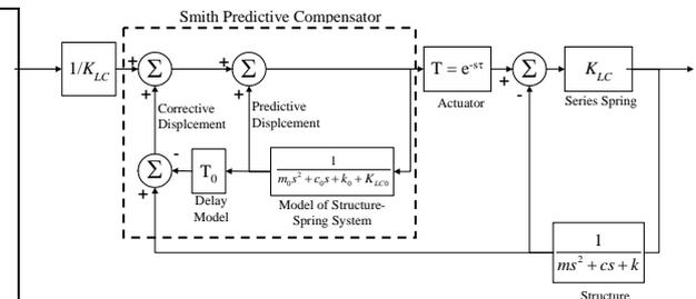
Figure 9. Smith predictive time-delay compensator
