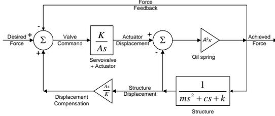
**Figure 2:** Force control of [3] rearranged.
