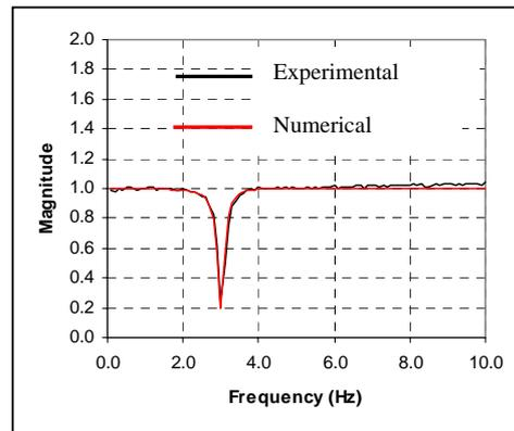
Figure 8. Magnitude of the input force - output force frequency response function
