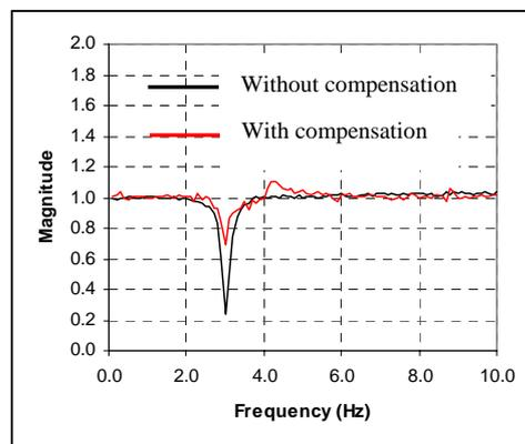
Figure 10. Magnitude of the input force - output force frequency response function
