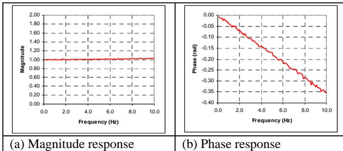
Figure 7: Frequency response function of the actuator in displacement control
