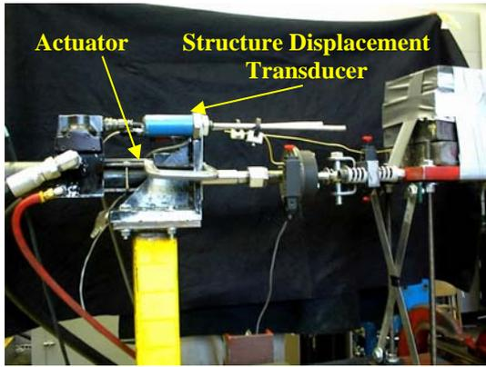
Figure 6: (b) Small scale actuator detail
